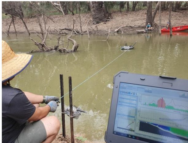
Mapping channel complexity and flow habitat with a Acoustic Doppler Current Profiler
