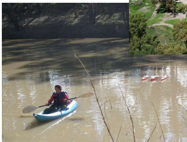
Sara Shaeri Karimi recording flow and bathymetric data with an Acoustic Doppler Current Profiler (Baaka) River, June 2021
