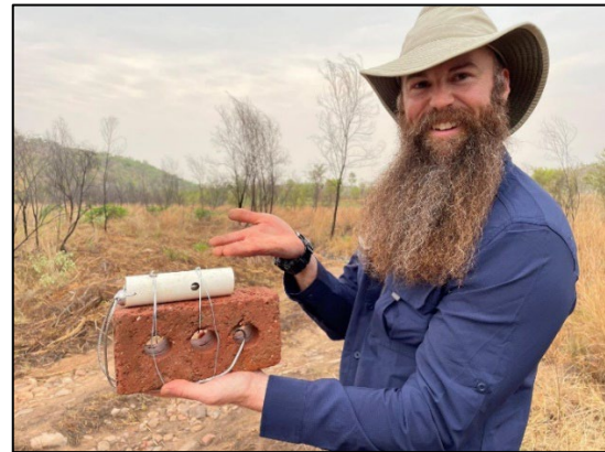
DBCA's David Chemello (East Kimberley District) and Michael Venarsky surveying waterbirds on Lake Kununurra (left), Mike with a pressure transducer to be installed in a dry creek bed (right)
